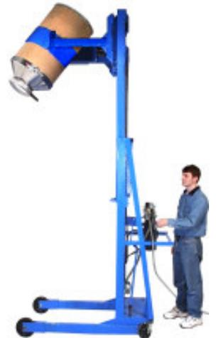
Special 185 Series Below-Hook Kontrol-Karriers are available with longer arms to provide the increased clearance required for rotating a drum with cone attached.
