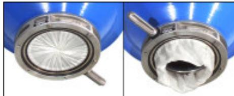
**Iris Valve** with aluminum body for controlling the flow of fine and coarse materials. The operator revolves the handle around the valve to open and close the flexible sleeve. A wide range of fine to coarse materials can be handled without clogging the iris valve.
