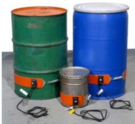
To attach to your drum, simply wrap the drum heater around and attach the spring and hook arrangement. Because these heaters are pliable, they conform to the wall of the drum. Though quick to fasten, they assure thorough band contact for effective heat transfer through the drum wall to the material inside. They are more flexible than metal band heaters, and therefore able to conform to the drum's surface to transfer heat more effectively.
