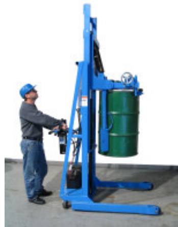
2. Raise your drum. Use MORStak to lift your upright or horizontal drums from the floor.
