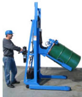
3. Tilt your drum to horizontal, then transport it to the desired location.
