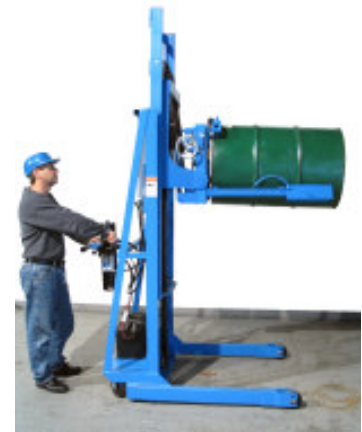
4. Release the clamp, then raise your drum to place it on a rack up to 8.5 feet high on a 4-tier rack.
