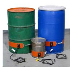
To attach to your drum, simply wrap the drum heater around and attach the spring and hook arrangement. Because these heaters are pliable, they conform to the wall of the drum. Though quick to fasten, they assure thorough band contact for effective heat transfer through the drum wall to the material inside. They are more flexible than metal band heaters, and therefore able to conform to the drum's surface to transfer heat more effectively.
