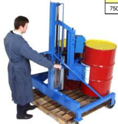
Roll the Pallet-Server to the side of the pallet. Pivot the lifting mechanism to the left or right to reach a drum in any position on the pallet. Use the Pallet Server to lift your drum clear of the pallet. You can pick or place all four drums, one at a time, with acces from only one side of the pallet.
