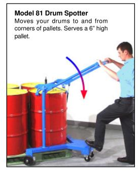
This ergonomic drum palletizer is equipped with battery powered lift for ease of use. Approach the corner of a pallet to push the jaws below the rim of your drum, then use the single control to raise it. The jaws automatically grip the drum rim on the way up. Set the drum down, and the jaws release when the weight is removed.
